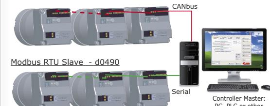
Drives control through commands by Master Controller. Suitable for multi axes systems (up to 127 drives). Built in powerful Motion Module functionalities, assures perfect synchronization among axes and reduces Master Controller workload.
