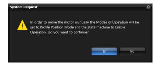
This window appear because with these type of drives, in order to do a motor movement using direct commands, it is required to be in 'Profile Position Mode'.
