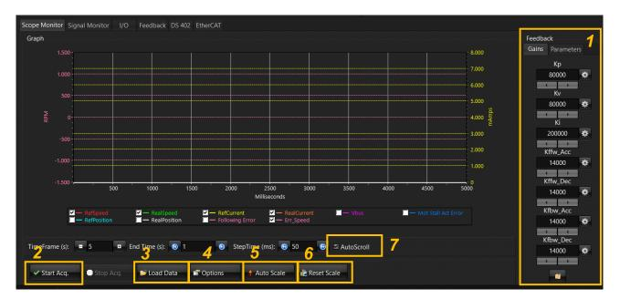
It also permit to modify **Gains and Parameters** (1) used in Feedback Modality, to find the better conditions.
