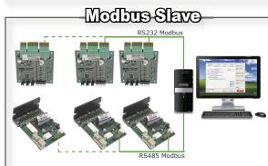
Through the serial interface is possible to control the motor position, rotation speed and control all the hardware resources of which this 'open frame' drives are equipped. For example, it is possible a check of the digital or analog I/O, or monitor the drive operating status.
