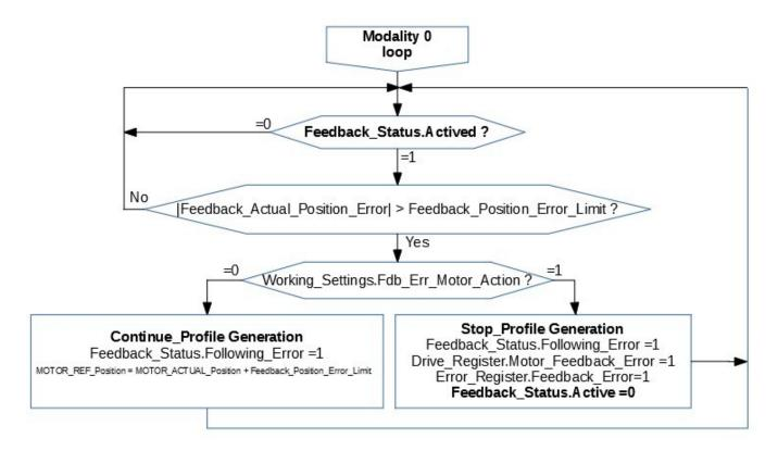
The *Drive\_Register.Motor\_Feedback\_Error*, can go to 1 also if least one of the bit (1,3,5,8) of the *Feedback\_Status* object is 1.
