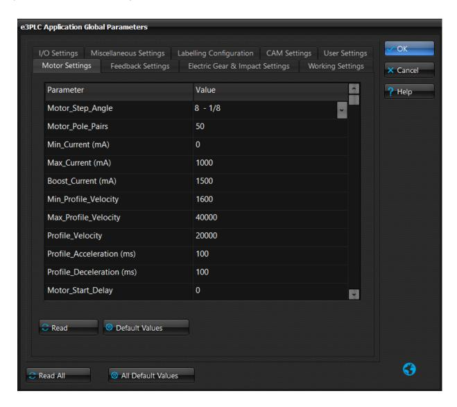
The parameter values will be stored together with the application instruction in the e3PLC application file (.plc). It is possible to read or write all the parameters (Read All / Write All buttons) from the drive or only the parameters of a single category (Read / Write) to the concerning drive.
