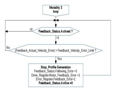
The *Drive\_Register.Motor\_Feedback\_Error*, can go to 1 if least one of the bit(1,3,5,8) of the *Feedback\_Status* object is 1. When the bit *Drive\_Register.Motor\_Feedback\_Error* is ON, the Close loop is disabled and at the motor is supplied the current defined with the object *Min\_Current*.
