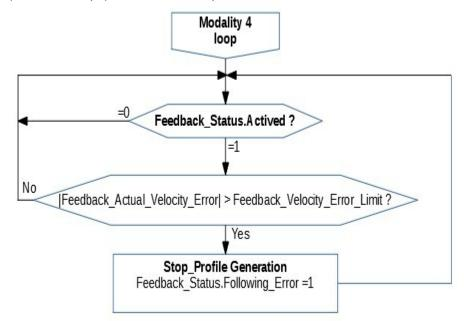
The *Drive\_Register.Motor\_Feedback\_Error*, can go to 1 if least one of the bit(1,3,5,8) of the *Feedback\_Status* object is 1. When the bit *Drive\_Register.Motor\_Feedback\_Error* is ON, the Close loop is disabled and at the motor is supplied the current defined with the object *Min\_Current*.
