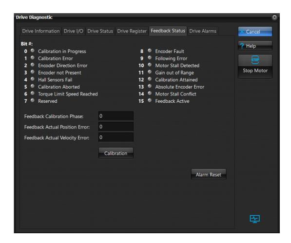
The Calibration procedure it's necessary to align the encoder mounted on motor rear shaft at the stator position. Are available two Calibration Procedure:
