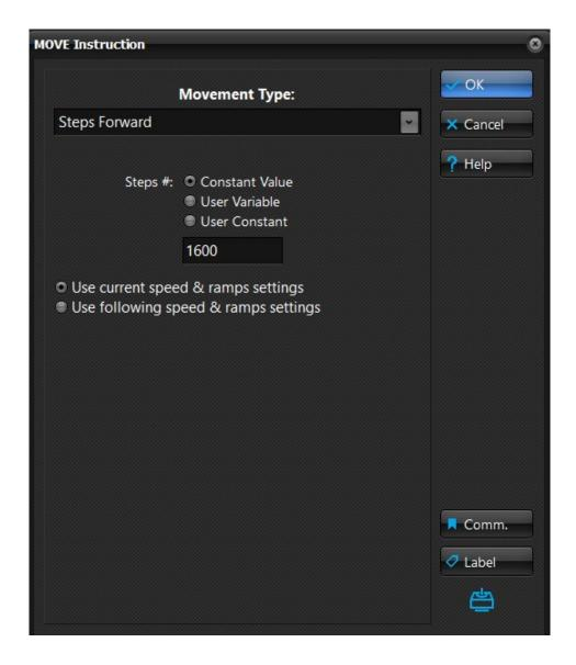
When the 'Use current speed & ramps settings' radio button is checked the motion profile is given by the current values of the motion parameters.
