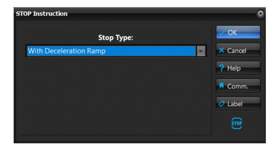
The stop types with Trigger Input or with Sync Object act in the same way as the movement types (see § 8.3.3 and §8.3.4). The STOP instruction doesn't wait for the end of the movement before passing the execution to the next application instruction. To wait until the motor movement is completed it is necessary to insert a WAIT for motor into the standstill instruction just after the MOVE instruction.
