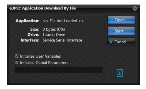
If the 'Initialize User Variables' checkbox is checked the User Variables initialization values set in the IDE (see §1.8) will be sent together with the user application, otherwise the current user variables values stored in the drive are retained.
