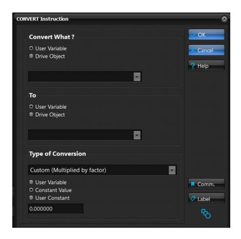
The CONVERT instruction is the only e3PLC instruction that perform the calculation using the floating point (REAL) arithmetic. Thus even though the conversion result is converted to an integer (losing the decimal part), the source user variable and the conversion factor (user variable or constant value) can be REAL type.
