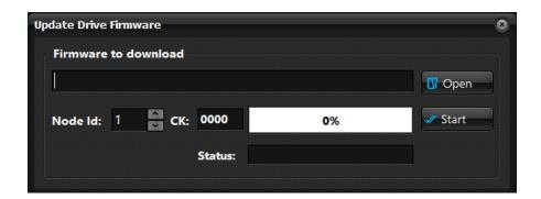
!! The firmware update is a critical process that could makes the drive unusable !! Perform this operation only under EVER supervision.
