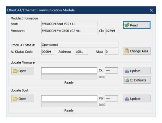
Pressing the 'Change Alias' button it is possible to select a different station Alias. The new setting will be active at the next drive switch-on.
