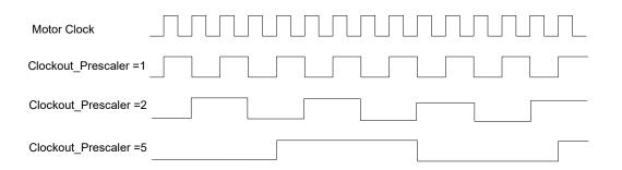
The Motor Clock Frequency depend on the motor speed and *Motor\_Step\_Angle* object so for example if the motor runs at the speed of 200 rpm we have :
