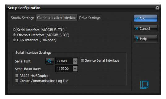
If the Baud Rate, Drive Nodeld and Drive Model are not known it is possible to start a network scan by pressing on the 'Find' button:
