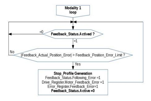
The *Drive\_Register.Motor\_Feedback\_Error*, can go to 1 also if least one of the bit (1,3,5,8) of the *Feedback\_Status* object is 1.
