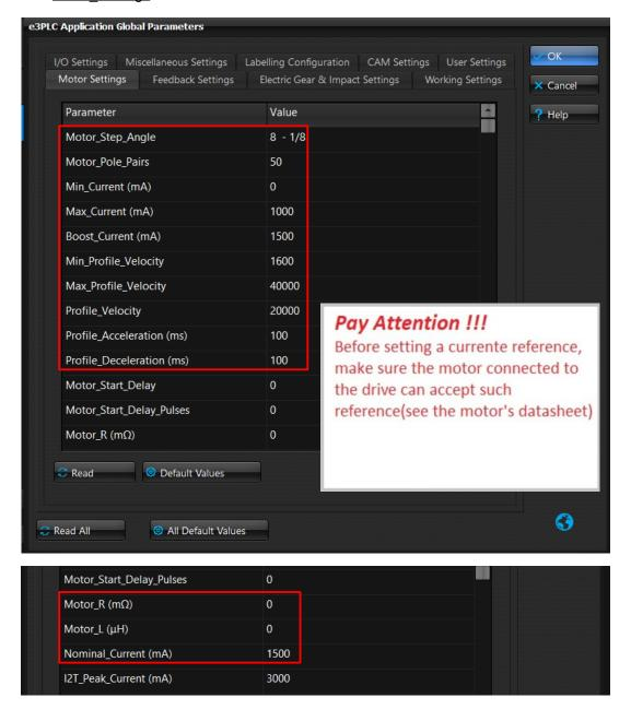
About the parameters Motor\_R and Motor\_L, it's possible omitted the value if it's enabled the automatic motor parameters detection. (bit *Drive Working Settings.Motor RL Detetection* =1).
