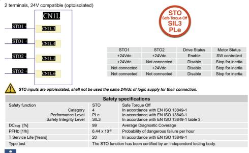
Refer to the "Safety Manual\_STO on SW5-AW5 Series" for more details of the Safe Torque Off function characteristics.
