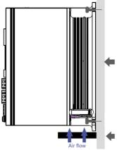
Aluminium dissipating support 33 x 30.5 cm min 0.5 thickness min
