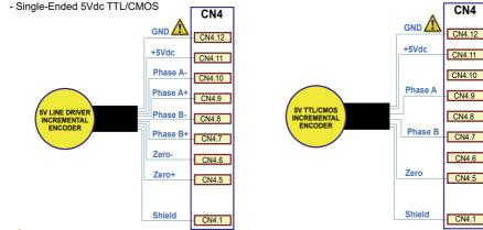
GND is internally in common with power ground, this is potentially dangerous. Take all necessary measures to avoid possible contacts in the final installation.
