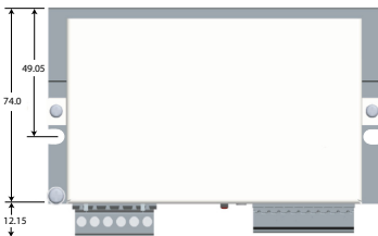
CN2: Digital inputs and output 10 position, pitch 3.81mm, PCB header connector
