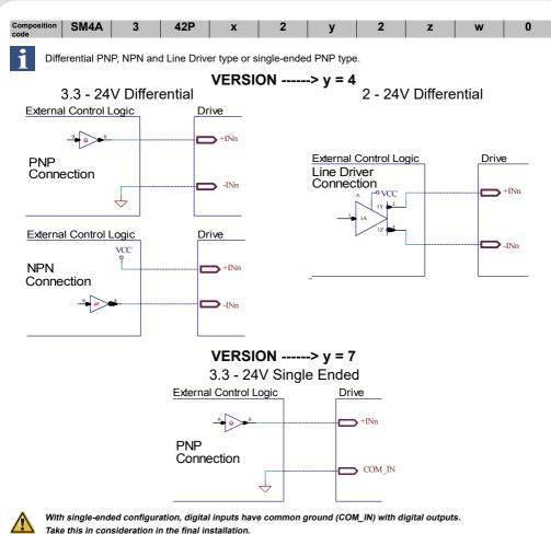
N.B. It's recommended to use 2Vdc digital inputs only in Differential Line-Driver configuration to have more noise immunity.
