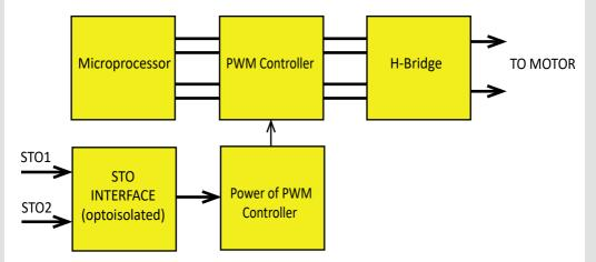
The drive has a safety feature that is designed to provide the Safe Torque Off (STO) function. Two inputs signlas are provided which, when not connected, prevent the upper and lower devices in the PWM outputs from being operated by the digital control core. This provides a positive OFF capability that cannot be overridden by the control firmware, or associated hardware components.
