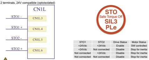
STO inputs are optoisolated, shall not be used the same 24 Vdc of logic supply for their connection.
