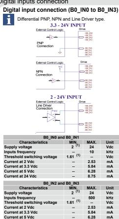
(1) N.B.: it's recommended to use 2 Vdc digital inputs only in differential Line-Driver configuration to have more noise immunity.
