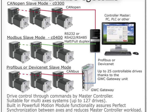
Drive control through commands by Master Controller. Suitable for multi axes systems (up to 127 drives). Built in Powerful Motion Module functionality assures Perfect Synchronization between axes and reduces Master Controller workload.
