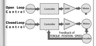
Better control compared to both an open loop stepper solution and a servo-controlled brushless solution
