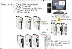
Drive control through commands by Master Controller. Suitable for multi axes systems (up to 127 drives). Built in powerfull Motion Module functionality assures perfect synchronization among axes and reduces Master Controller workload
